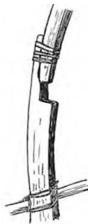
Fig. 148. Men's house roof spar binding, Păpítălăi .
